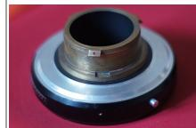
Mitchell 35R: 3 off,  $\frac{1}{4}$ " wide prongs on a 42mm barrel. Flange focal distance = 56mm measured to sl prongs. Overall clearance between lens mount and gate = 42mm. The prong next to a locking slot is n Lenses: Super Baltars and Kowa. Picture shows a Hasselblad to 35R adapter. Likely early 35R camera
